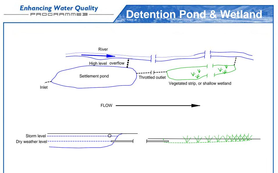
Concept of planned installation at Mains of Balgavies, to intercept a main field drain
