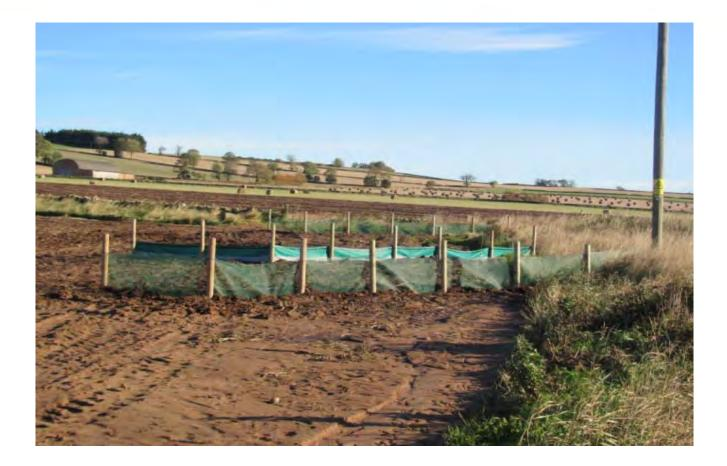
Filter fences B (furthest away, coarse filter), C (fine filter) and D (nearest, coarse filter)
